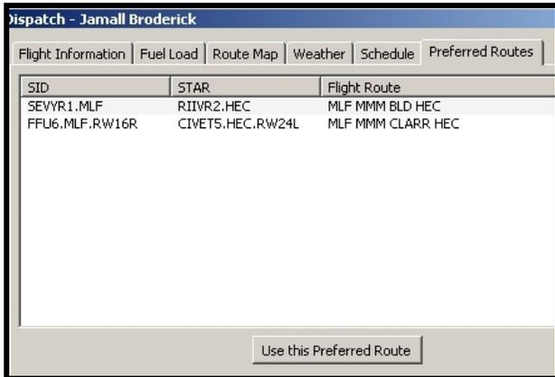
The preferred route is immediately recognized. The Dispatcher then accepts the preferred route. This is where they must do their homework. In the case of Salt Lake City (KSLC), you can't use the Sevr1 SID for southbound operations. The Dispatcher then adjusts your fuel levels, so that you have enough juice to get to your preferred destination, and then neatly packages it up and sends to you.
